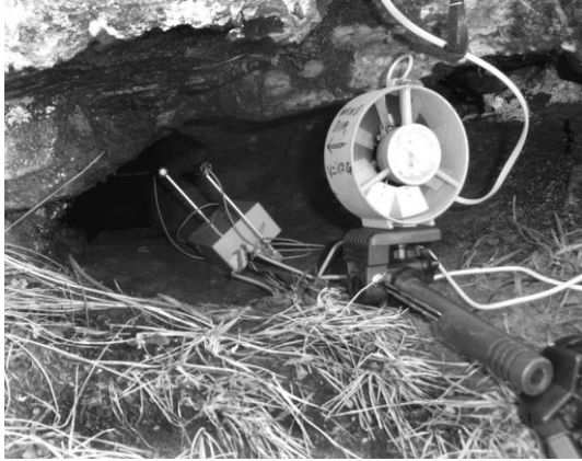
Figure 2. An ultrasonic anemometer (left) and a mechanical anemometer (right) recording data are located in the bat access hole to measure the rate of air flow.
