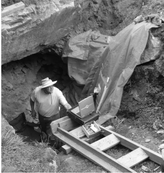
Figure 5. A tarp was fastened to one side of an excavation to cover an area where air was passing through a zone of rocks. Cardboard was taped to the tarp to provide a rigid surface and a hole was cut in the cardboard and tarp. An anemometer was placed in this hole where the air flow was then concentrated.
