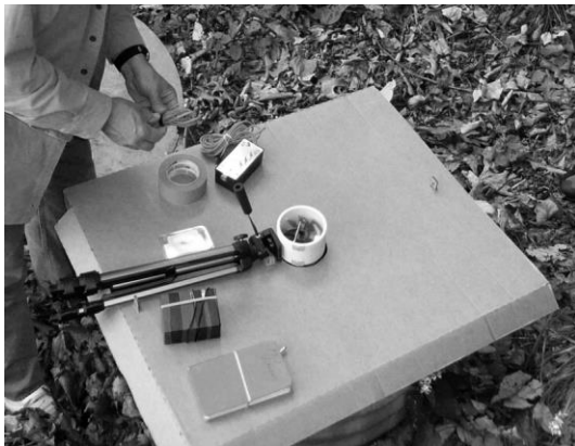
Figure 4. Cardboard has been placed over the entrance (a vertical culvert pipe) to Basswood Cave. The anemometer placed over a hole in the cardboard records the rate of air flow.
