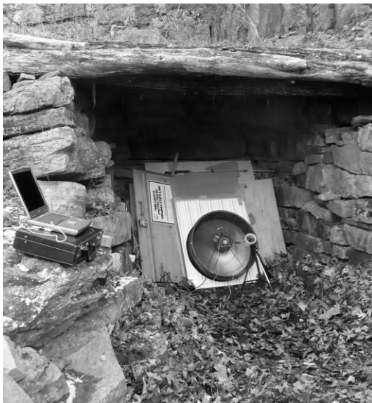
Figure 1. The rectangular doorway Butler Cave’s Sofa entrance has been sealed around a fan. The fan blows alternately in and out of the cave in even intervals. A signal is sent from the fan to a recording data logger when the fan changes direction.
